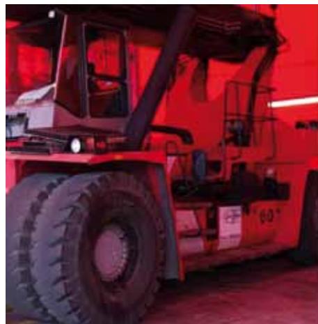
Picture of the left side of the Kalmar reach stacker cockpit, showing limited space for LNG tank positioning
