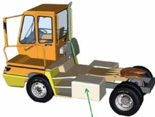
Hydraulic tank, battery and air compressor moved to the same side
