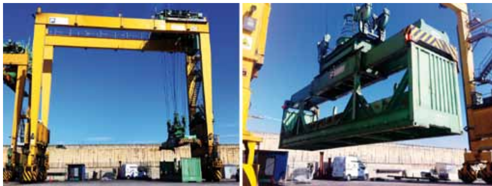
Figure 42. RTG Operating with 15L Displacement Gen-Set
