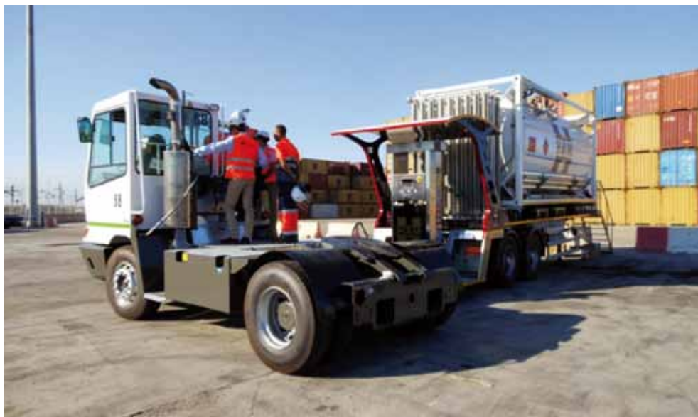
Figure 39. LNG Terminal Tractor Prototype at Noatum Container Terminal Valencia
