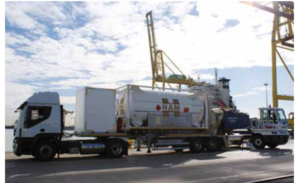
Figure 38. Mobile LNG Supply Fuel Station
