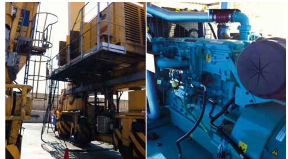
Figure 43. Tests of the 15L Gen-Set on RTG at NCTV
