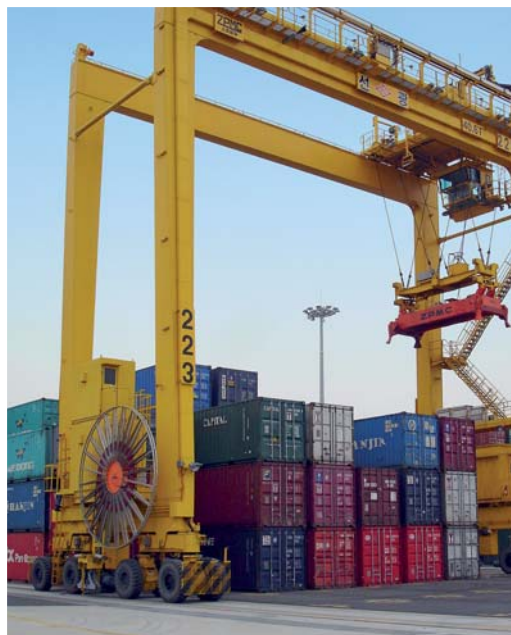
RTG Electrification with the Motorized Cable Reel System or the Conductor Bar System - by Conductix-Wampfler
