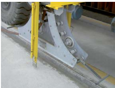
A special “wide” cable guide is used, designed to accommodate lateral movements of the RTG
