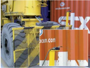
Safety devices at the front and rear of the crane prevent accidental collisions with misaligned containers
