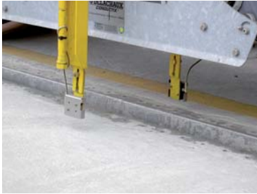
Since there are no guiding beams, two optical sensors , one on each side of the trench, control the travel deviation of the crane
